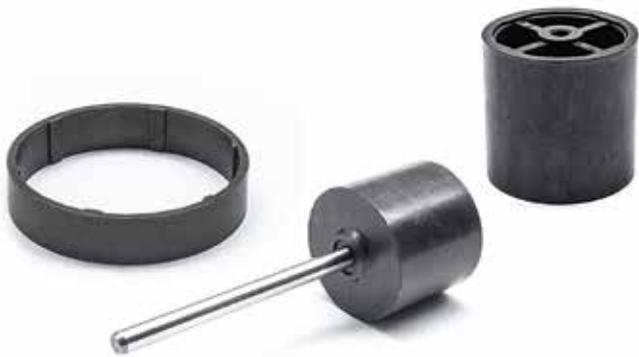
Multipolar anisotropic magnets are produced in molds with integrated multipolar or radial magnetic field for particle aligning during processing in injection molding.
